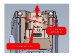
• The SAM need to be inserted on the reverse side of the module
